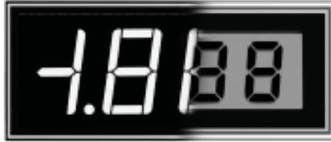
Backlit LCD displays should be used if the meter is to be operated in both high and low-light conditions. Murata Power Solutions uses reliable, long-life LEDs as the light source in all of our backlit LCD meters. A “B” suffix added to the end of the Murata Power Solutions model number specifies a backlit model.
