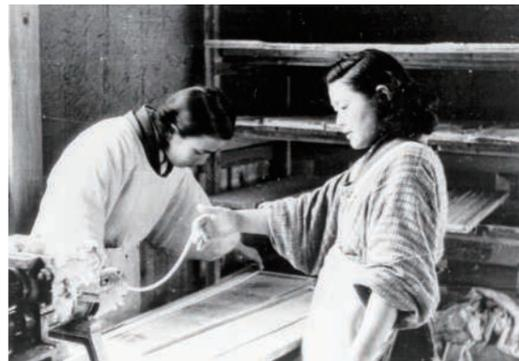
Production of titanium-dioxide ceramic capacitors
