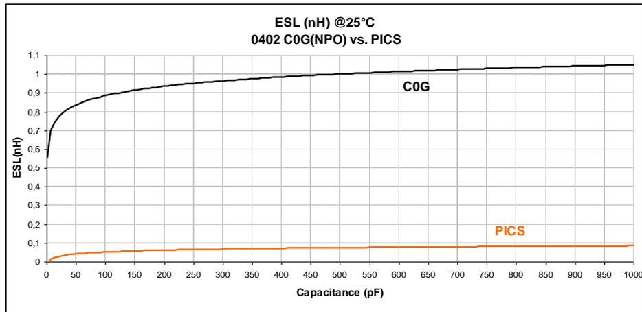
Fig.5 Comparison between 0402 C0G (NPO) and PICS capacitors
