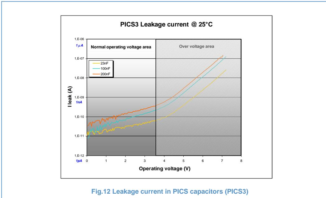
Fig.12 Leakage current in PICS capacitors (PICS3)
