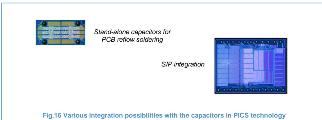
Some stand-alone capacitors with a JEDEC compatible footprint (0805, 0603, 0402, 0201, 01005...) are available and can be customized under request.
