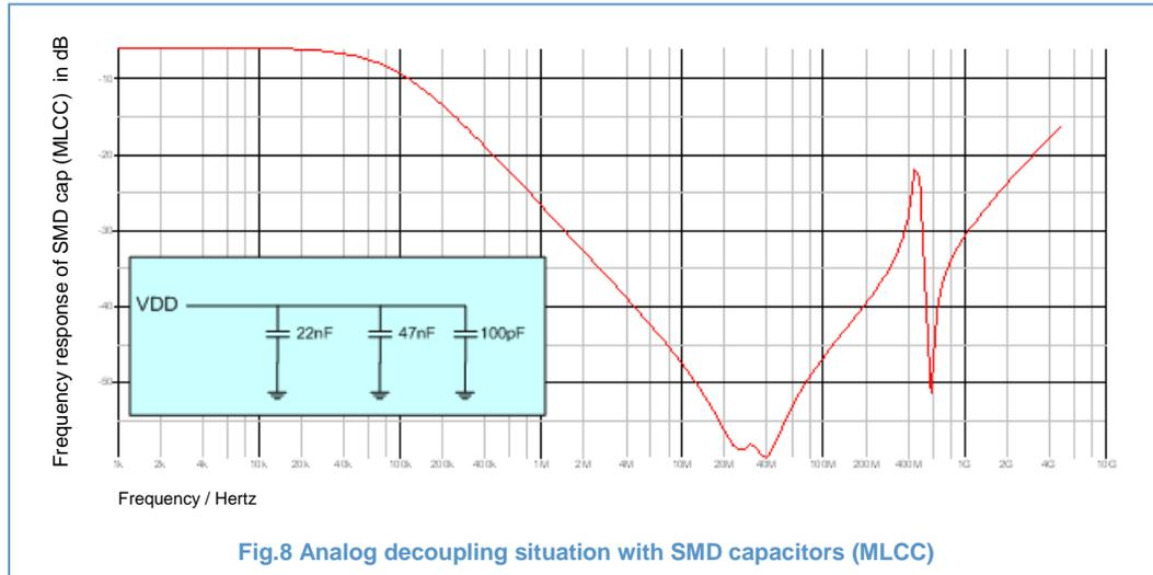
For such a situation, the decoupling capacitors value needs as a first order to stay at the same value (no optimization). The advantage with PICS is a better efficiency at the resonance frequencies (lower ESR).
