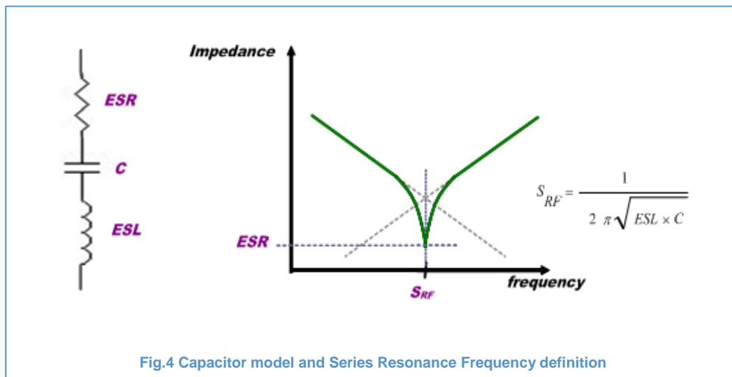
Both ESR and ESL are lowered compared to MLCC and Tantalum capacitors for the same capacitance value, having a direct impact on the applications performances.
