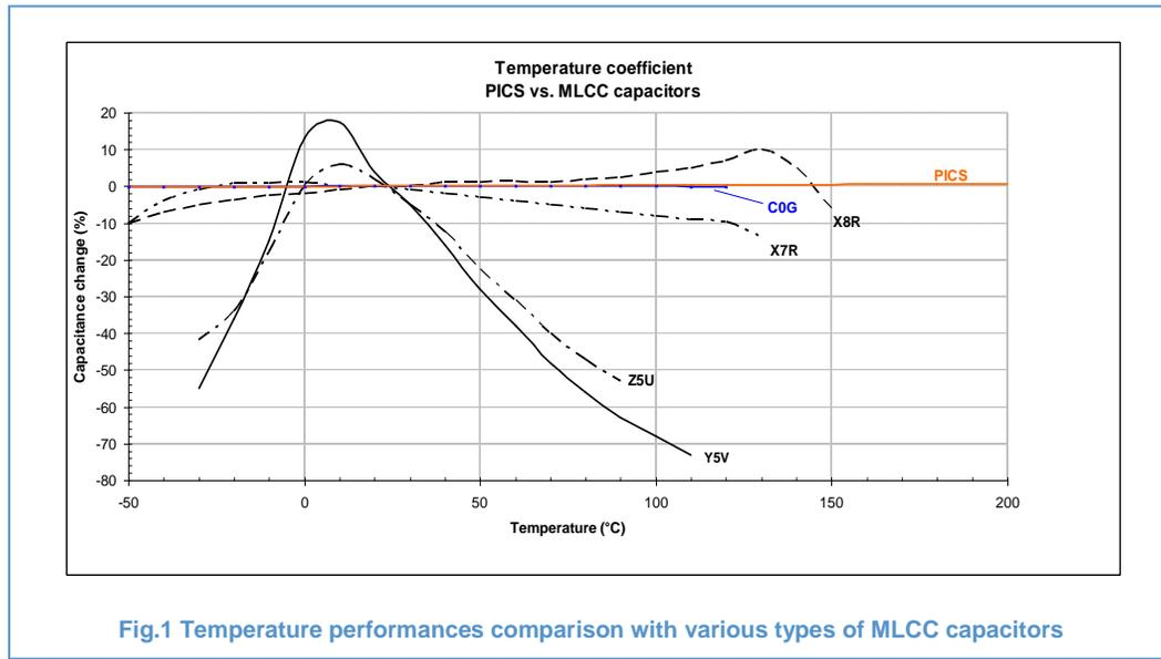
Fig.1 Temperature performances comparison with various types of MLCC capacitors
