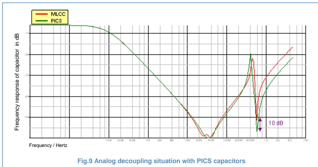
Note that the PICS technology allows fine tuning of the ESL to place the notches at the required frequencies.
