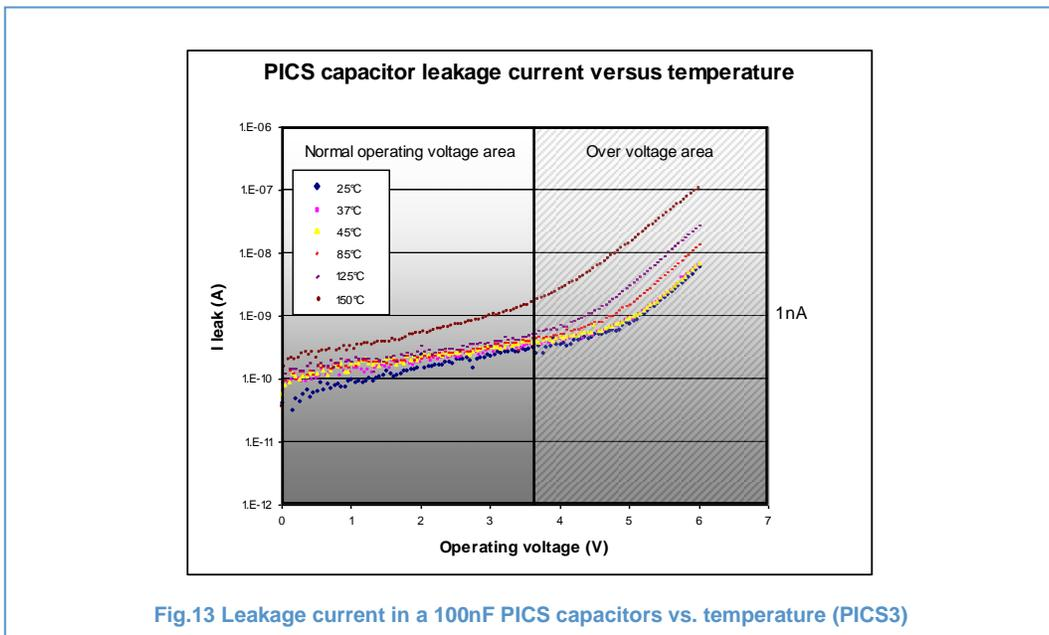
Fig.13 Leakage current in a 100nF PICS capacitors vs. temperature (PICS3)
