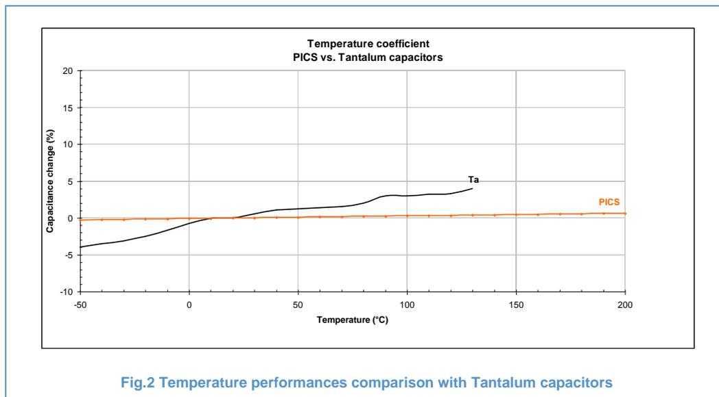
Fig.2 Temperature performances comparison with Tantalum capacitors
