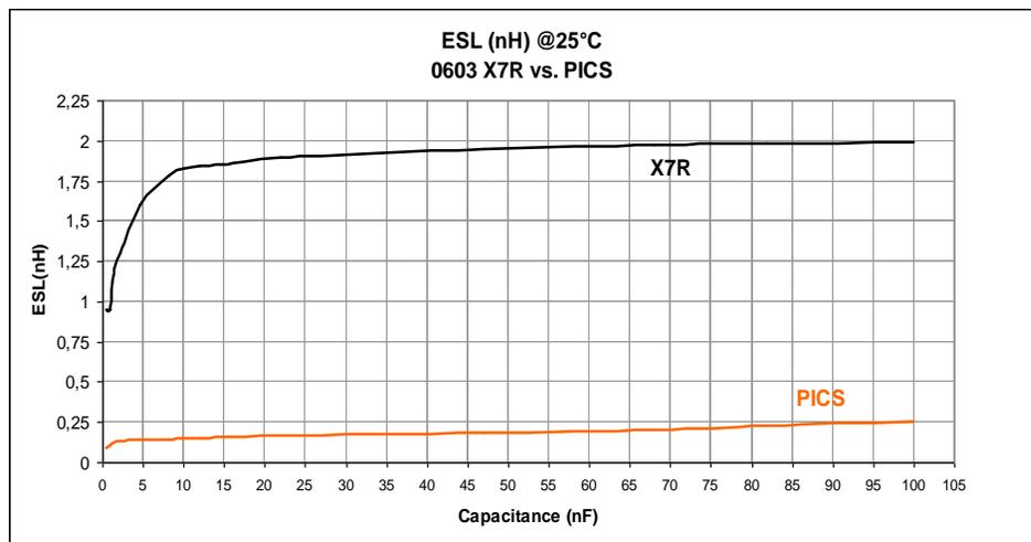
Fig.6 Comparison between 0603 X7R and PICS capacitors
