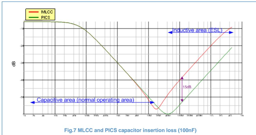
The insertion loss at the resonance frequency is directly driven by the capacitor ESR (lower with PICS technology). The decoupling efficiency can be improved by 15dB in the inductive area.
