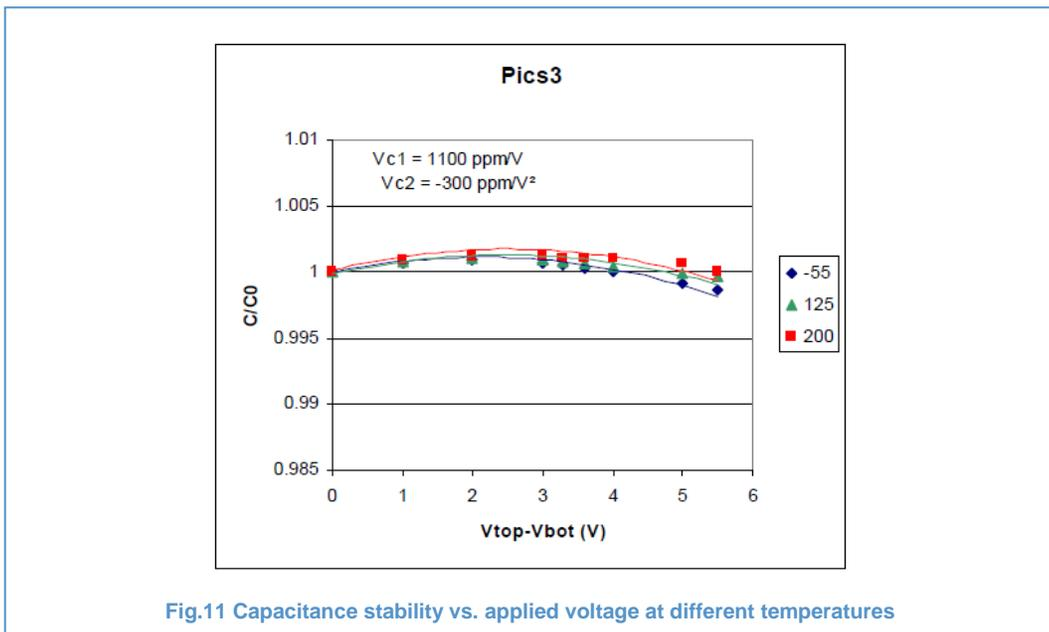
Fig.11 Capacitance stability vs. applied voltage at different temperatures
