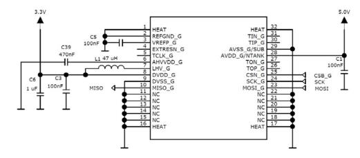
Figure 8. SCR1100 recommended circuit diagram.
