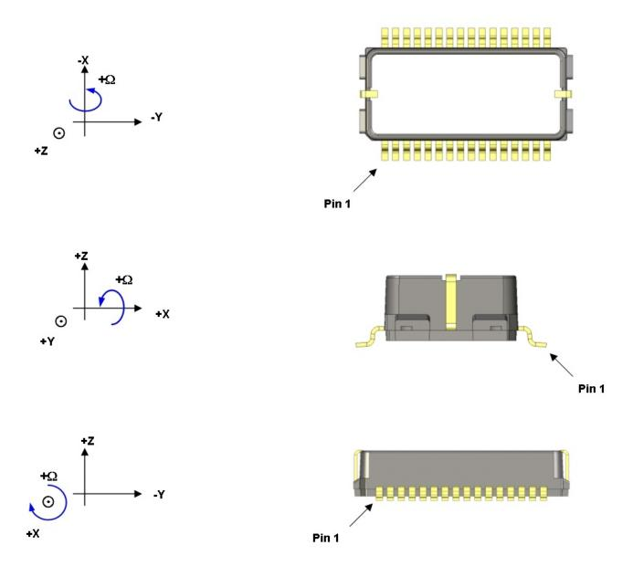
Figure 12. SCR1100 angular rate measurement direction.
