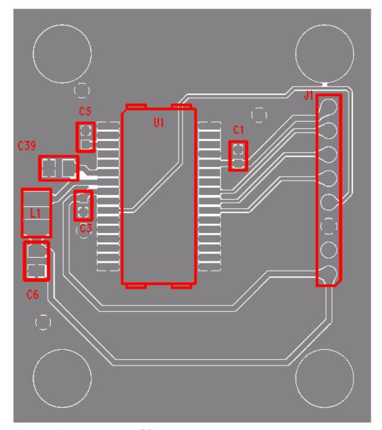
Figure 11. Example layout for SCR1100.
