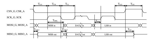
Figure 3. Timing diagram of SPI communication
