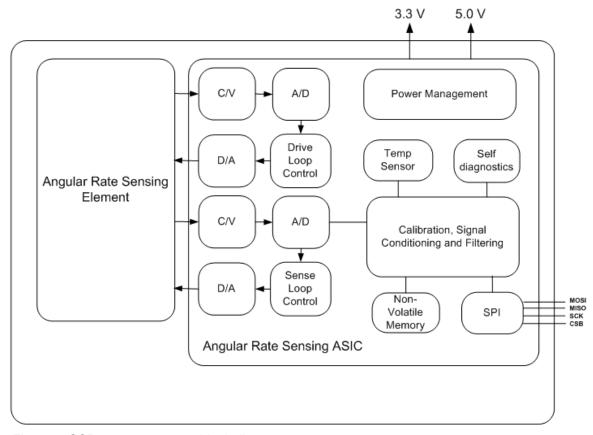
Figure 1. SCR1100 component block diagram.
