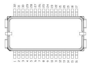
Figure 7. SCR1100 pinout diagram.
