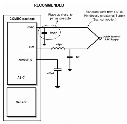
Figure 10. Layout recommendations for DVDD\_G/LHV pin decoupling.
