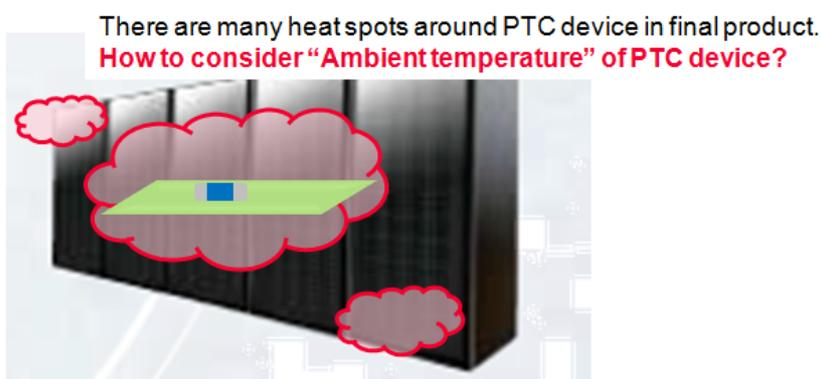
**Figure 2.5 Surrounding condition of PTC device in final products**
