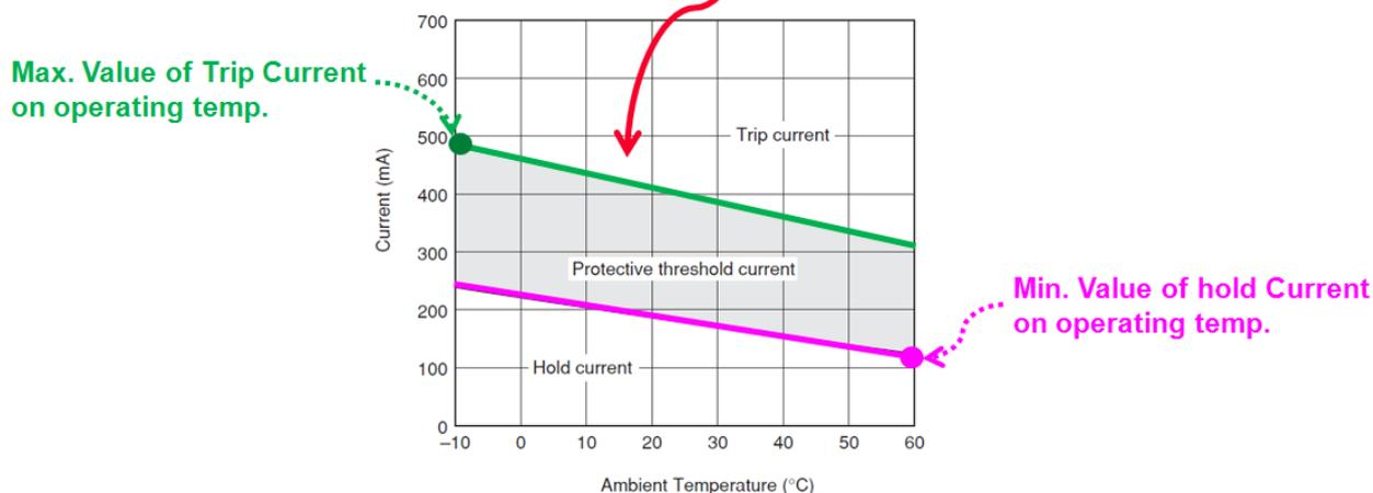
Figure 2.4 Selection process of Hold-current and Trip-current (ex. PRG21BC3R3-type)
