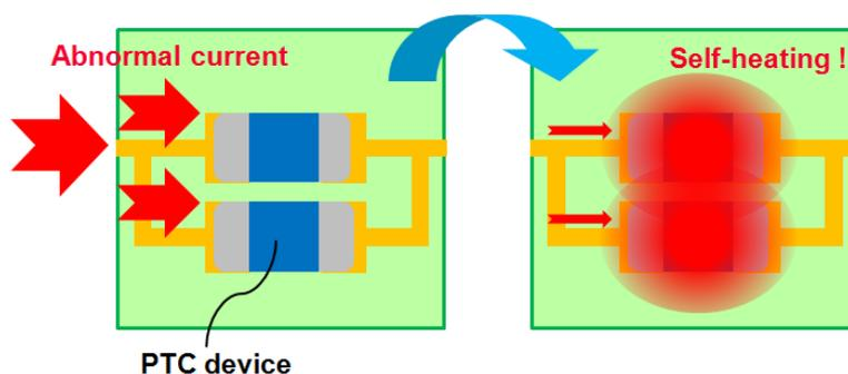
**Figure 2.7** Each PTC device gives heating-up to each other
