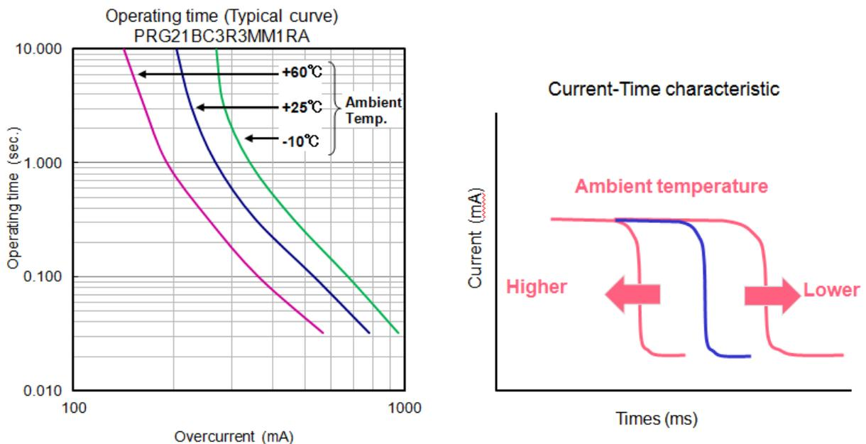
**Figure 2.10** Time trip operation is depending on ambient temperature
