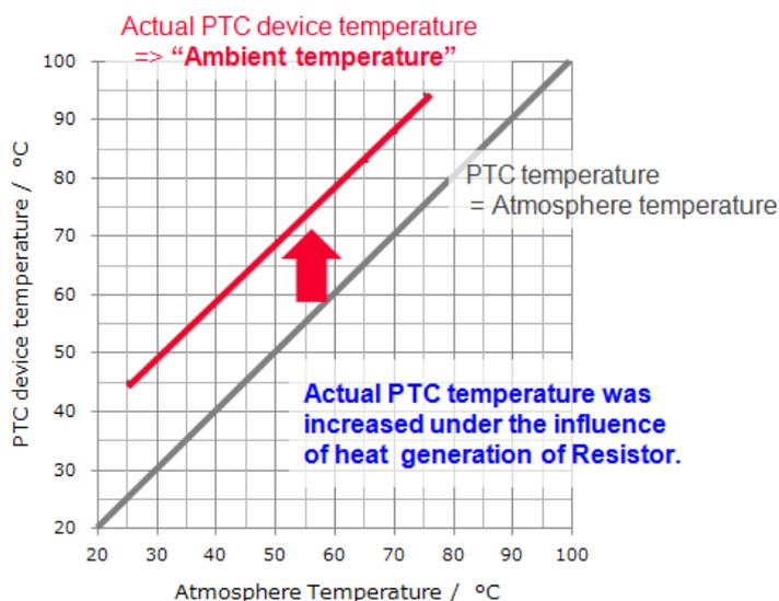
**Figure 2.6 Actual PTC device temperature and Atmosphere temperature**
