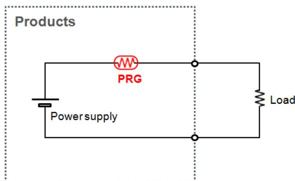
Figure 2.1 Basic circuit using PTC device
