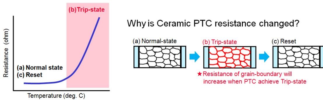
**Figure 1.1 PTC temperature-resistance characteristic and its origin**
