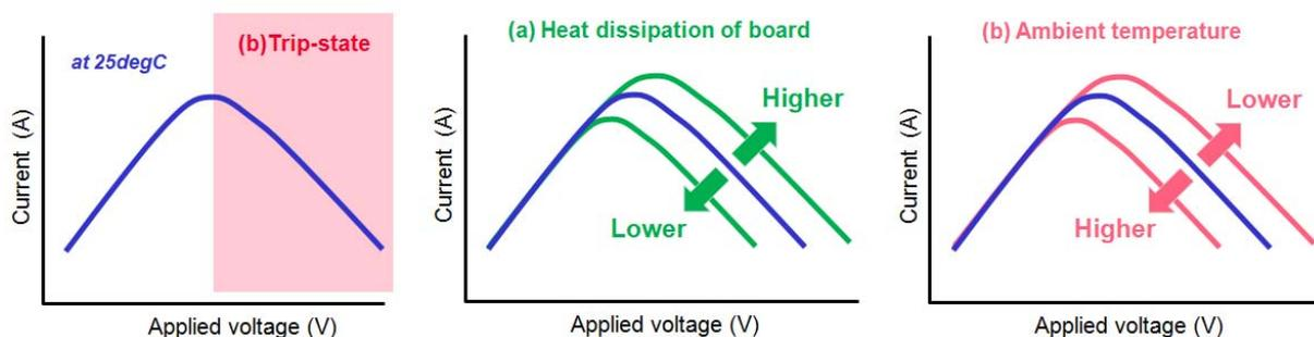
**Figure 1.2 Current-Voltage, and it is depending on Heat-dissipation and Ambient-temp.**
