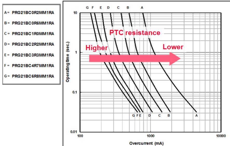
**Figure 2.9** Time trip operation is depending on individual PTC resistance
