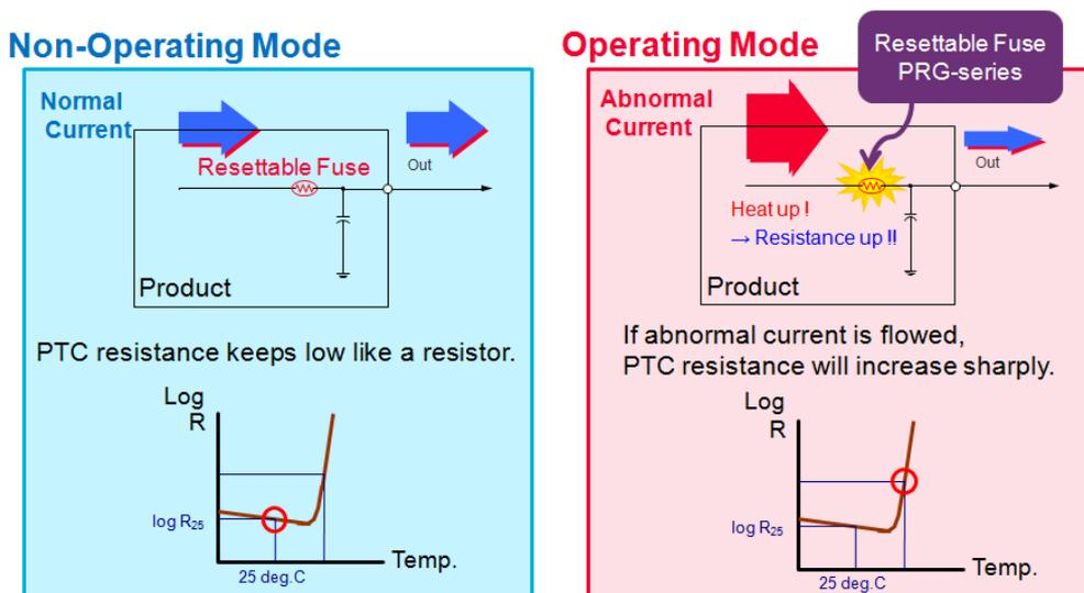
Figure 2.2 Operation of PTC device
