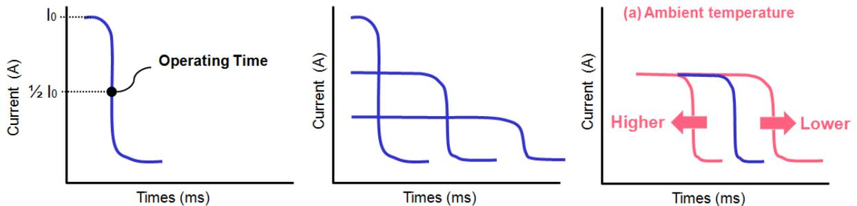
**Figure 1.3 Current-Time characteristic**
