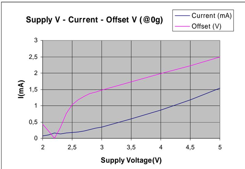
Figure 1. Low Supply Voltage and Power Consumption
