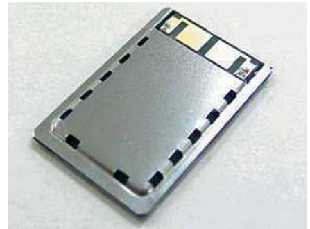
Fig. 2: External appearance of the VSLBP1913E Series rectangular piezoelectric speaker
