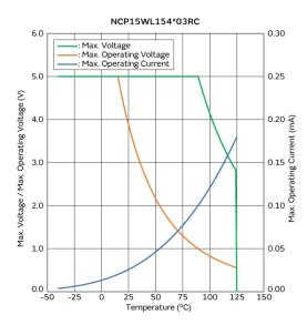
Max. Voltage, Max. Operating Voltage/Current **Reduction Curve**
