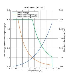
Max. Voltage, Max. Operating Voltage/Current Reduction Curve
