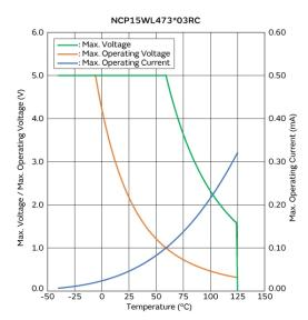
Max. Voltage, Max. Operating Voltage/Current **Reduction Curve**
