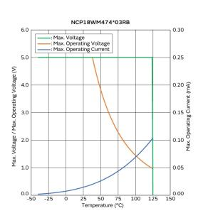
Max. Voltage, Max. Operating Voltage/Current Reduction Curve
