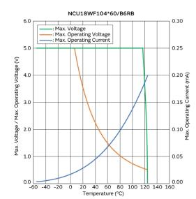
Max. Voltage, Max. Operating Voltage/Current Reduction Curve
