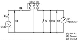
R1+Rg=R2=470Ω ±5%, Rg=50Ω C2=10pF (Including stray capacitance and Input capacitance of RF Voltmeter) E1: S.S.G. Output voltage
