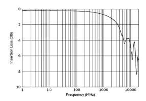
Common Mode Insertion Loss Characteristic (Typical Value)
