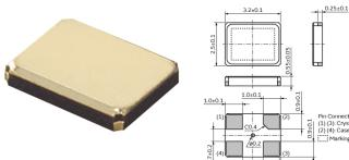
Pin Connection (1) (3): Crystal Ter (2) (4): Case GND (in mm) Note: This datasheet may be out of date. Please download the latest datasheet of XRCJH13M000F1QA0P0 from the official website of Murata Manufacturing Co., Ltd.
