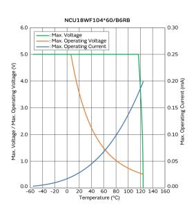
Max. Voltage, Max. Operating Voltage/Current Reduction Curve
