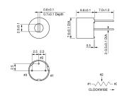
unit : mm Tolerance : ±0.3 Note: This datasheet may be out of date. Please download the latest datasheet of PV12P201A01B00 from the official website of Murata Manufacturing Co., Ltd.
