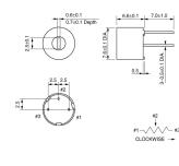
unit : mm Tolerance : ±0.3 Note: This datasheet may be out of date. Please download the latest datasheet of PV12P504A01B00 from the official website of Murata Manufacturing Co., Ltd.
