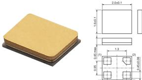
1.3 (2) (1) Crystal Terminal (2) No Connect (3) Crystal Terminal (4) GND (in mm) Note: This datasheet may be out of date. Please download the latest datasheet of XRCGD48M000K1Q01R0 from the official website of Murata Manufacturing Co., Ltd.
