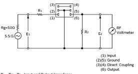
R1 + Rg = R2 =Input and Outout Impedance E1: S.S.G. Output Voltage
