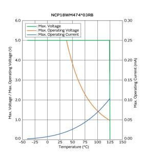
Max. Voltage, Max. Operating Voltage/Current Reduction Curve
