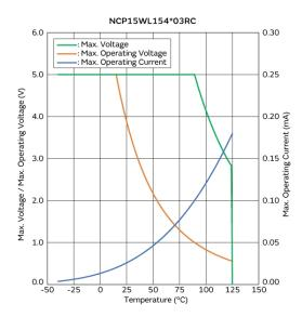
Max. Voltage, Max. Operating Voltage/Current **Reduction Curve**
