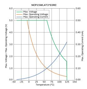
Max. Voltage, Max. Operating Voltage/Current **Reduction Curve**
