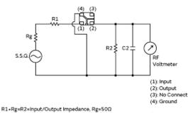
22-10pF (including stray capacitance and input capacitance of RF Voltmeter) E1: S.S.G. Output Voltage
