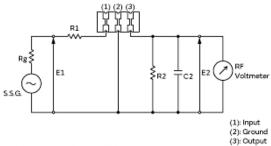
R1+Rg=R2=1000Ω ±5%, Rg=50Ω C2=10pF (Including stray capacitance and Input capacitance of RF Voltmeter) E1: S.S.G. Output voltage
