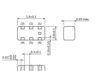
(1): Unbalance Port (2): GND (or DC Feed) (3)(4): Balance Port (5)(6): GND
