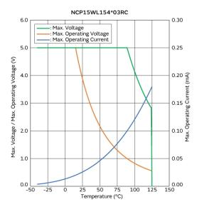
Max. Voltage, Max. Operating Voltage/Current **Reduction Curve**
