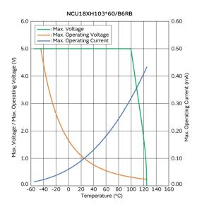
Max. Voltage, Max. Operating Voltage/Current **Reduction Curve**
