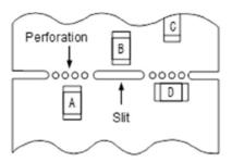
(3) Mounting components near screw holes
