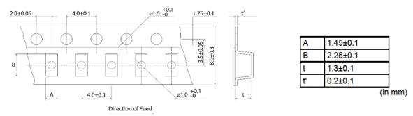
\* The dimensions of the cavity are measured at its bottom.
