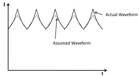
Current waveform when an inductor having poor characteristics is used for the required bias current characteristics
