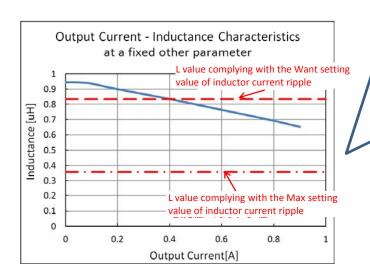
Change of the inductance value when the output current is changed
