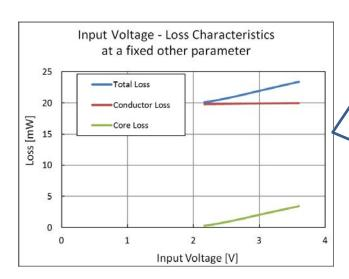
Changes of loss when the input voltage of a DC-DC converter is changed
