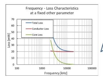
Changes of loss when the switching of a DC-DC converter is changed
