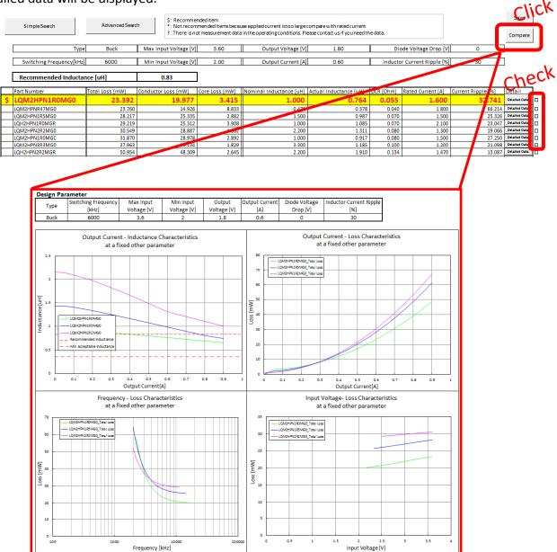
The above graph shows that LQM2HPN1R0MG0 is the most suitable inductor in this example.
