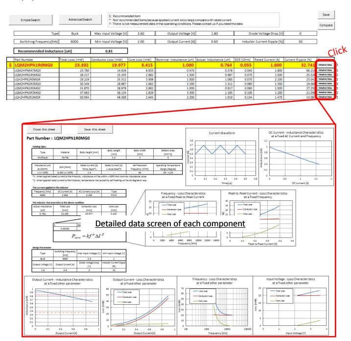
The data required to select inductors, from the basic catalog specifications to graphs of the characteristic fluctuations assuming actual use, will be displayed collectively in one sheet.
