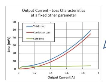
Changes of loss when the output current of the DC-DC converter is changed
