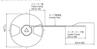
The tape for transducer shall be wounded clockwise.
