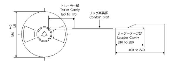
The tape for transducer shall be wounded clockwise. The feeding holes shall be to the right side as the tape is pulled toward the user.
