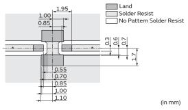
$^{\ast}$  Line width to be designed to match 50  $\Omega$  characteristic impedance, depending on PCB material and thickness.
