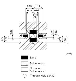
$^{*}$  Line width to be designed to match 50  $\Omega\,$  characteristic impedance, depending on PCB material and thickness.
