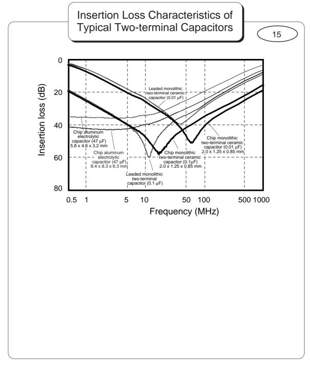
The above drawing shows examples of insertion loss measurements of typical capacitors. For leaded capacitors, the insertion loss is measured with the lead wires cut to 1 mm.
