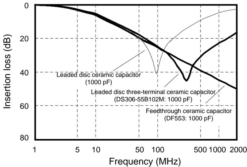
Feedthrough capacitors have a structure in which the ground electrode surrounds the dielectric and the signal terminal goes through the dielectric. Feedthrough capacitors are used by making a mounting hole in the shielding case and soldering the ground electrode directly to the shielding case (plate). Since this type of capacitor has no residual inductance on the ground terminal side as well as on the signal terminal side, it can provide nearly ideal insertion loss characteristics.
