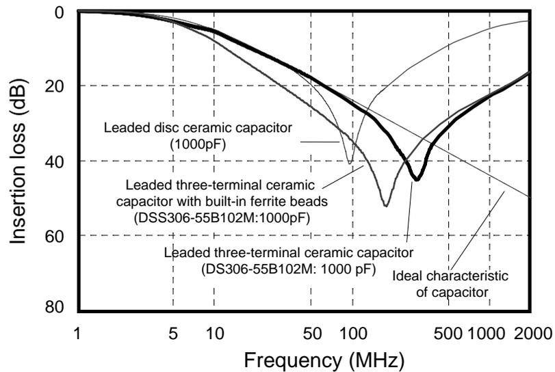
With leaded two-terminal capacitors, the residual inductance is larger because the lead wires work as inductors.
