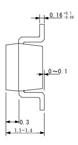
Coplanarity: less than 0.1mm(includiong under reflow condition)
