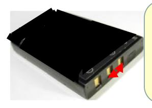
If a terminal shortcircuits, NTC and IC may be broken!
