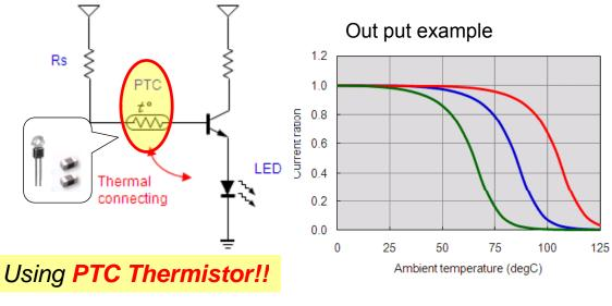
★ LED thermal protection: No need any IC but PTC Thermistor. **★** Current de-rating curve can be changed by different PTC products.
