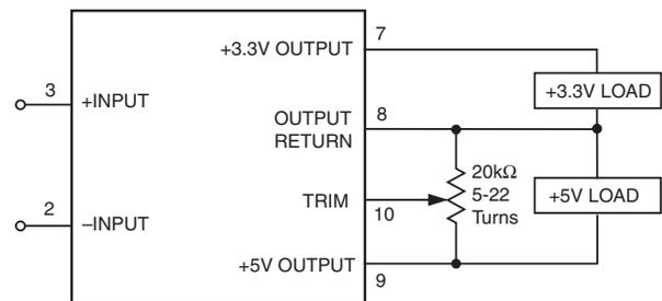
Figure 3. +5VOUT Trim Connections Using A Trim Pot
