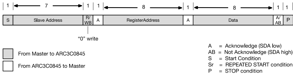
Figure 62: “Write” Data Transfer Format in Standard, Fast, Fast-Plus Modes
