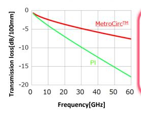
Having superior characteristics in the millimeter wave band, MetroCirc™ can differentiate itself from other products.
