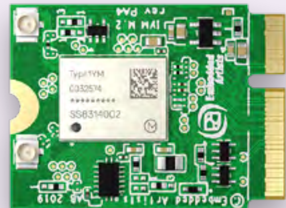
Type 1YM Dual band Wi-Fi® 11a/b/g/n/ac 2x2 MIMO + Bluetooth® 5.2
