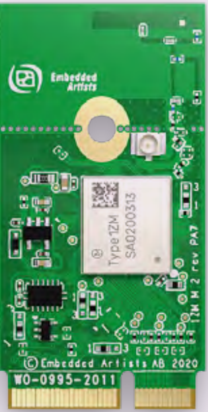
Type 1ZM Dual band Wi-Fi® 11a/b/g/n/ac + Bluetooth® 5.1
