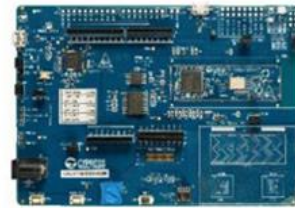
CY8CKIT-064B0S2-4343W PSoC™ 64 Secure Boot MCU (2 MB Flash, 1 MB SRAM), AIROC™ CYW4343W Murata 1DX module
