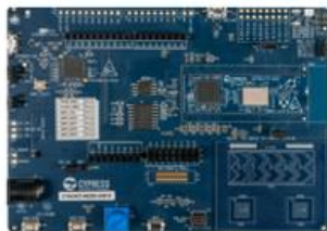
CY8CKIT-062S2-43012 PSoC™ 62 MCU (2 MB Flash, 1 MB SRAM), AIROC™ CYW43012 Murata 1LV module
