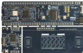
CY8CPROTO-062S3-4343W PSoC™ 62 MCU (512 KB Flash, 256 KB SRAM), AIROC™ CYW4343W Murata 1DX module
