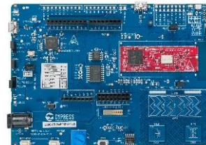
CY8CKIT-064S0S2-4343W PSoC™ 64 Standard Secure - AWS MCU (2 MB Flash, 1 MB SRAM), AIROC™ CYW4343W Murata 1DX module
