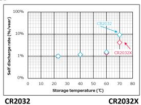
Fig.1 Self-discharge rate at each temperature CR2032 vs CR2032X
