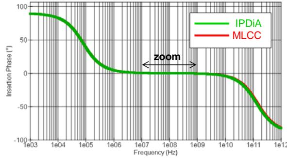
Figure 9: IPDiA Silicon Capacitor & MLCC models insertion phase (°)
