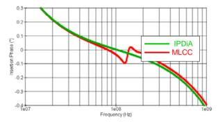
Figure 10: IPDiA Silicon Capacitor & MLCC models insertion phase (zoom)
