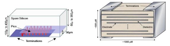
Figure 3: IPDiA Silicon Capacitor & MLCC simplified 0402 SMD construction
