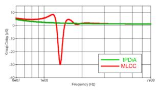
Figure 11: IPDiA Silicon Capacitor & MLCC group delay (pS)
