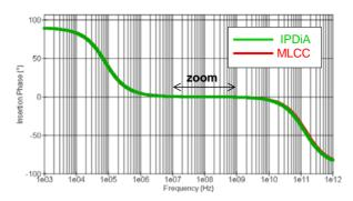
Figure 9: IPDiA Silicon Capacitor & MLCC models insertion phase (°)
