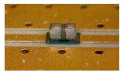
Figure 2: Silicon capacitor used as SMD compared with MLCC SMD
