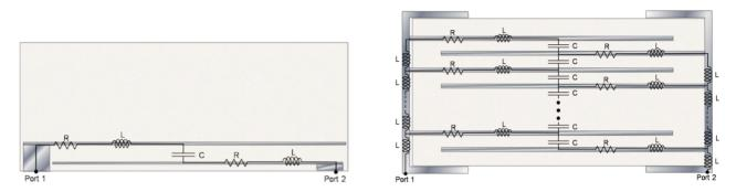
Figure 4: IPDiA Silicon Capacitor (left) & MLCC (right) simplified electrical parasitics related to technologies
