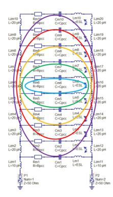
Figure 6: MLCC intrinsic multiple resonant frequencies
