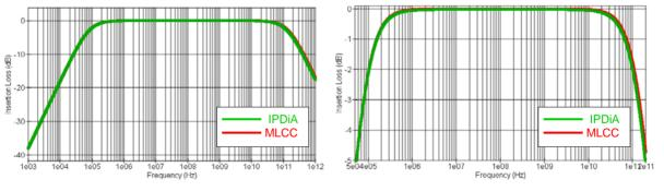
Figure 7: IPDiA Si Cap & MLCC models insertion loss (dB) Figure 8: IPDiA Si Cap & MLCC models insertion loss (zoom)
