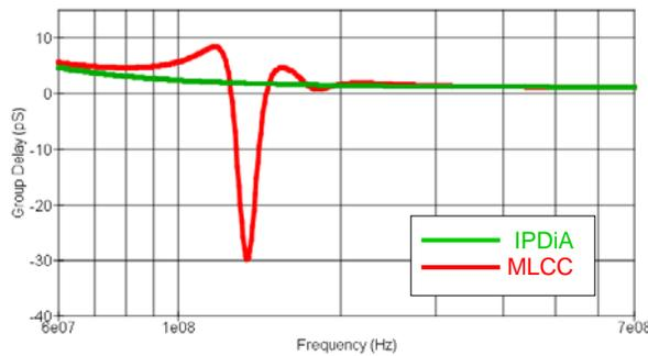
Figure 11: IPDiA Silicon Capacitor & MLCC group delay (pS)
