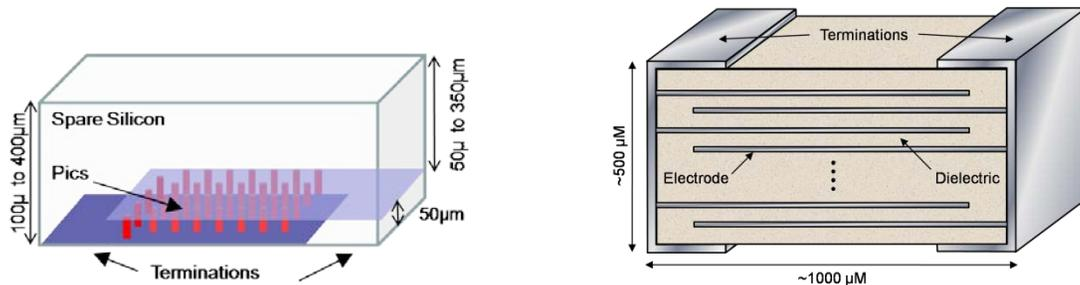
Figure 3: IPDiA Silicon Capacitor & MLCC simplified 0402 SMD construction
