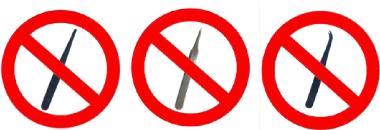
Figure 10: Example of tweezers unsuitable for picking up a die
