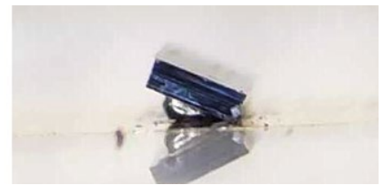
Figure 5 : Si-cap tilting examples, please note the solder excess
