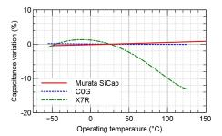
Fig. 1: Capacitance variation vs temperature (for UESL and MLCC technologies)
