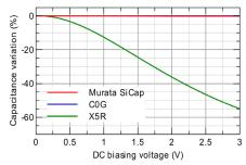
Fig. 2: Capacitance variation vs DC biasing voltage @ BV 5 (for UESL and MLCC technologies)
